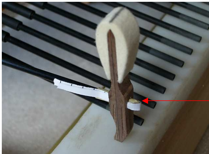
Fig. 16 Fit hammers on shank with travel paper
